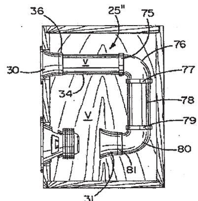
Fig. 13. Further refinement of modular port concept which uses port for cooling transducer. (From Gahm [12].)
