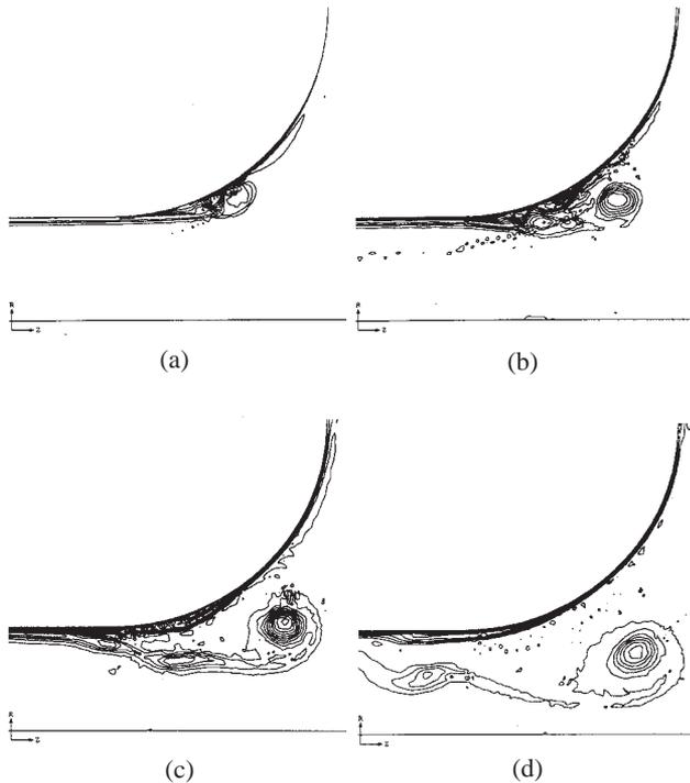
Fig. 7. Simulation of vortex shedding in highly radiused port on exit stroke. Note how early in the throat shedding begins. (From Roozen et al. [6].) (a)  $t = 7$  ms. (b)  $t = 9$  ms. (c)  $t = 11$  ms. (d)  $t = 13$  ms.
