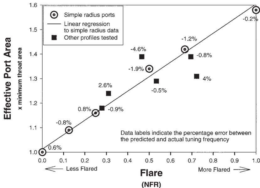
Fig. 30. Curve fit of flare rate to port tuning data.
