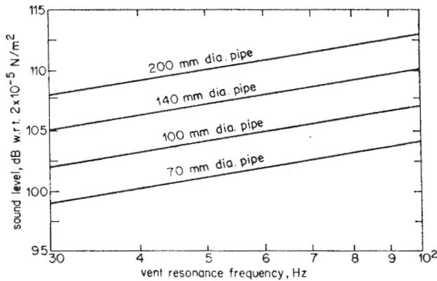
Fig. 5. Minimum SPL in a room of 2000 ft<sup>3</sup> (56.6 m<sup>3</sup>) for various-diameter long pipes and vent resonant frequencies before distortion is appreciable. Note that the larger the pipe, the better, and doubling the area improves performance by 10 dB. Also lower tuning requires a larger pipe. (From Harwood [1].)
