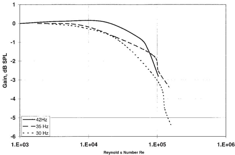
Fig. 24. Port compression versus Reynolds number in double 18-in (457-mm) subwoofer, 12 ft<sup>3</sup> (0.34 m<sup>3</sup>), tuned to 35 Hz with three straight round ports.
