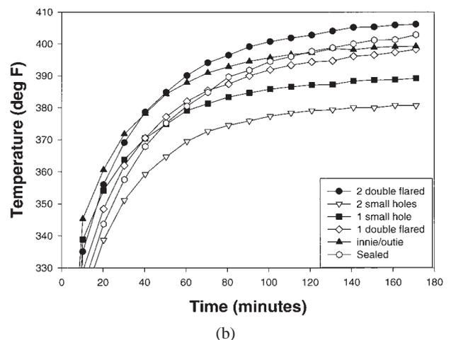
Fig. 53. Thermal repercussions for various port configurations versus time. (a) Box air temperature. (b) Voice-coil temperature.
