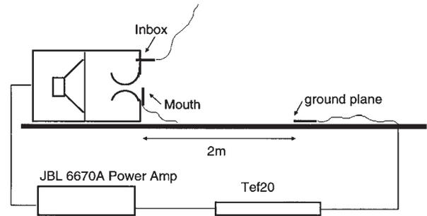
Fig. 31. Bandpass loudspeaker setup for compression testing. Before selecting the “in-box” position for all compression measurements, the three microphone locations shown were tried.
