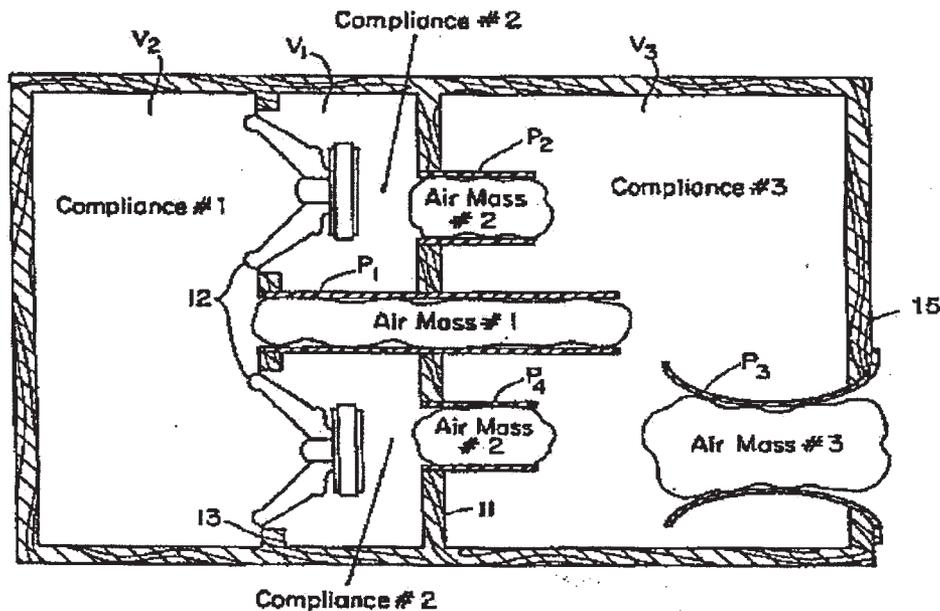
Fig. 9. Port 3 is shown with an elliptical cross section, which is said to be optimum. (From Gawronski and Caron [9].)
