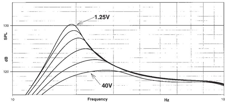
Fig. 33. Port compression measured in box for port with NFR = 0.25.
