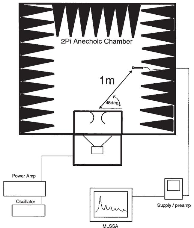
Fig. 38. Distortion measurement setup. A bandpass loudspeaker mounted in a  $2\pi$  anechoic chamber was used to measure distortion. Note off-axis position of microphone to avoid contaminating data with subsonic noise due to exit jets.
