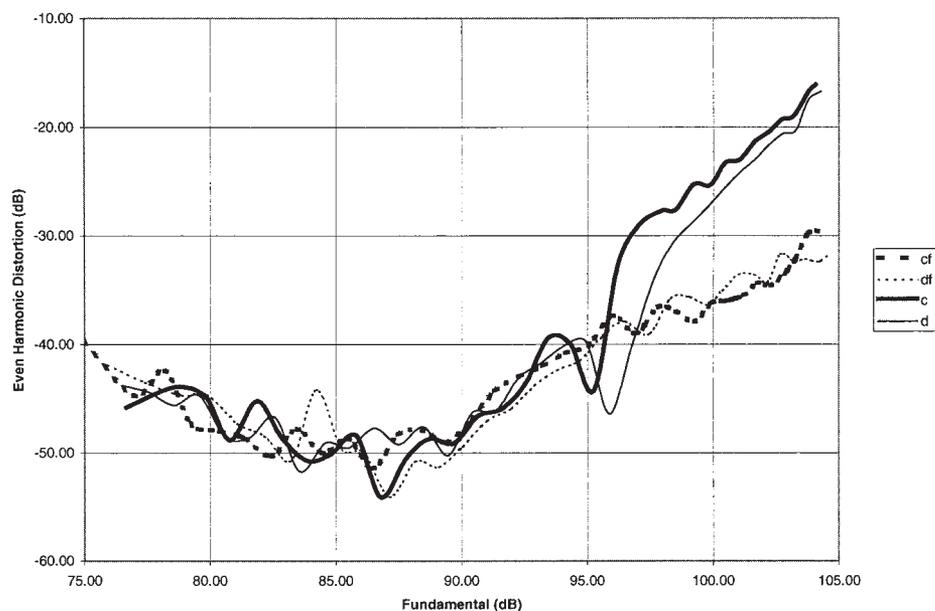
Fig. 51. Even harmonic distortion versus fundamental for ports cf (c with inside flange), df (d with inside flange), c, and d.
