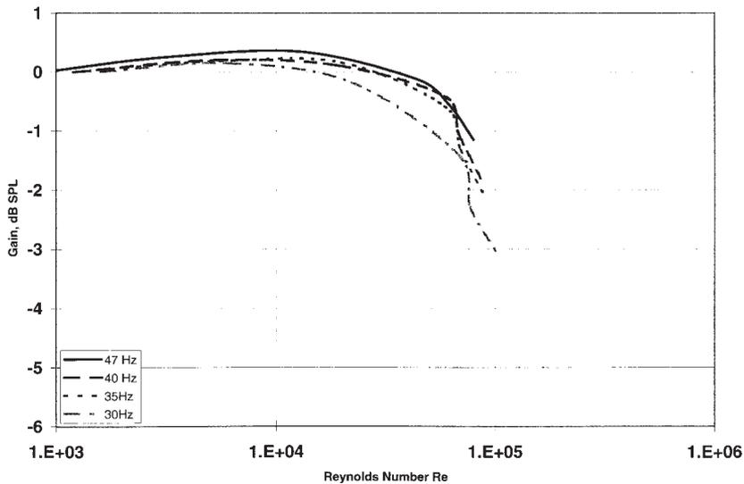
Fig. 25. Port compression versus Reynolds number in double 18-in (457-mm) subwoofer, 12 ft<sup>3</sup> (0.34 m<sup>3</sup>), tuned to 39 Hz with four straight square ports.
