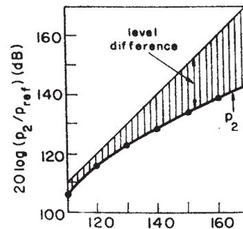
Fig. 2. SPL transmitted through an orifice in a plate as a function of driving sound pressure  $p_1$ . Shaded portion shows difference in level (compression) of  $p_1$  and  $p_2$ . (From Ingard and Ising [7].)
