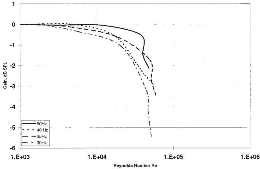
Fig. 23. Port compression versus Reynolds number in double 18-in (457-mm) subwoofer, 10 ft<sup>3</sup> (0.28 m<sup>3</sup>), tuned to 45 Hz with a single rectangular port.
