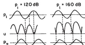
Fig. 4. Traces of pressure  $p$  and velocity  $u$  at low and high SPL in an orifice. At low SPL  $p_1$  and  $p_2$  are in quadrature; at high SPL they are in phase.  $p_1$  represents pressure from backside of cone;  $p_2$  is radiated sound from port. (From Ingard and Ising [7].)
