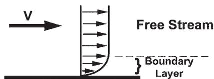
Fig. 18. Velocity profile near a stationary wall.
