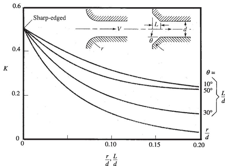
Fig. 27. Entrance loss coefficients for rounded and beveled inlets. Lower curve applies to rounded geometry.  $K$ —loss coefficient related to ratio of pressure drop to velocity. Note:  $r/d = 0.2$  yields a nearly lossless inlet. (From White [18].)
